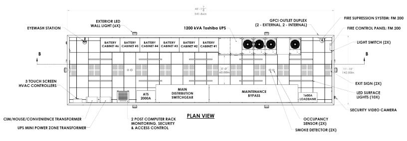
Noted above is a floor plan for a single UPS CIM from a top-down perspective with equipment labeled.
